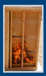
When siding catches fire, the flames can burn into the stud wall cavity at a lap joint, as shown in this test photo. When this occurs, the entire house can be lost to wildfire.
