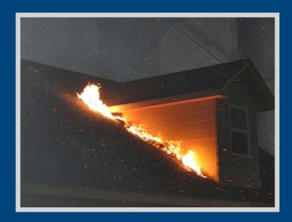
This test photo shows how burning debris at the intersection of the roof and walls exposes the wall to direct contact with flames once the debris is ignited by wind-blown embers.
